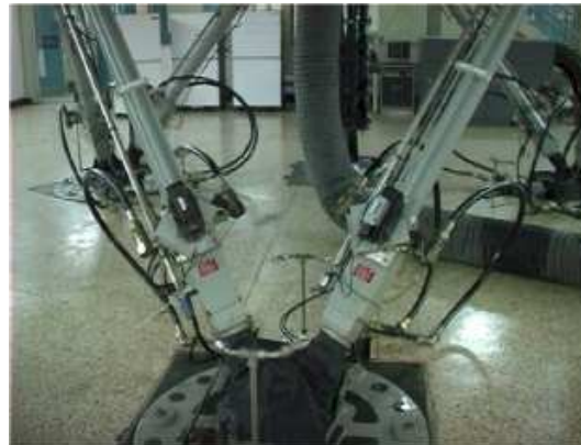
(b) A lower view of a 737 simulator that uses 60in jacks on a 6 DOF system.
