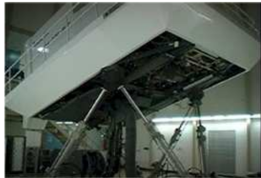
(b) To produce an acceleration and rotation cue this sim tilts upward sharply and moves forward on its haunches.
