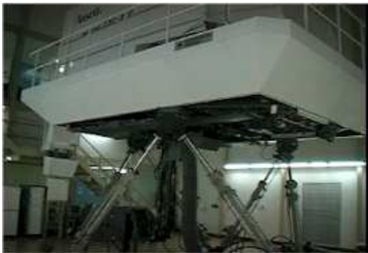
(a) A simulator producing a braking motion cue by slightly tilting forward.
