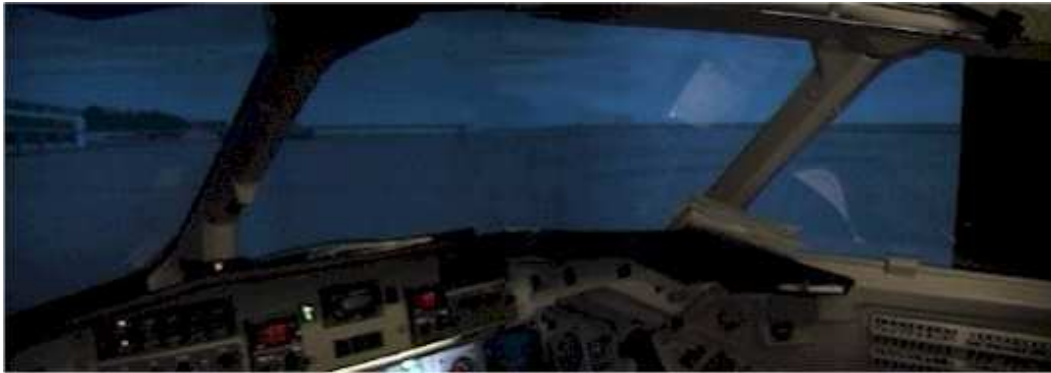
Figure 1.3: The cockpit of a SAAB 340 simulator using the latest in panoramic collimated displays. Notice the un interrupted view and cross cockpit viewing.
